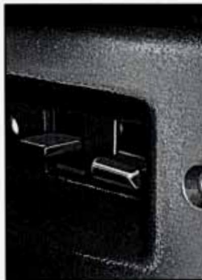
The switch is located on the front of the seat. To recline the seatback hold the switch up. Hold the switch down to raise the seatback.
