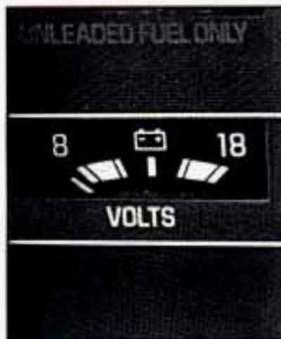
When your engine is not running, but the ignition is on (in the "Run" position), the gage shows your battery's state of charge in DC volts. When the engine is running, the gage shows the condition of the charging system. Readings between the red warning zones indicate the normal operating range.
