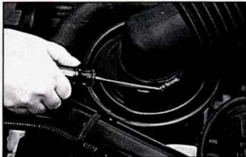
Your air cleaner is on the driver's side of the engine compartment. To check or replace the filter, use a screwdriver to loosen the hose clamp, then lift the rubber duct.
