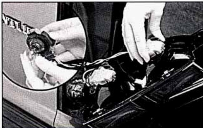
4. Press the bulb housing release lever and turn the housing 1/6 turn counterclockwise to remove it.
