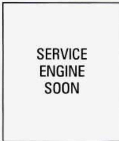
A computer monitors operation of your fuel, ignition and emission control systems. This light should come on when the ignition is on, but the engine is not running, as a check to show you it is working.
