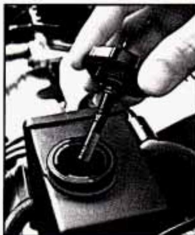
The power steering fluid reservoir is located on the passenger's side of the engine compartment.
